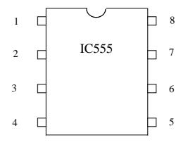
1 = Ground, 2 = Trigger, 3 = output, 4 = Reset, 5 = Control voltage, 6 = Threshold, 7 = Discharge, 8 = +Vcc
